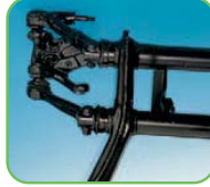
Front Axle Beam Assembly 65→LHD (needs converting)* For Vehicles with Discs
